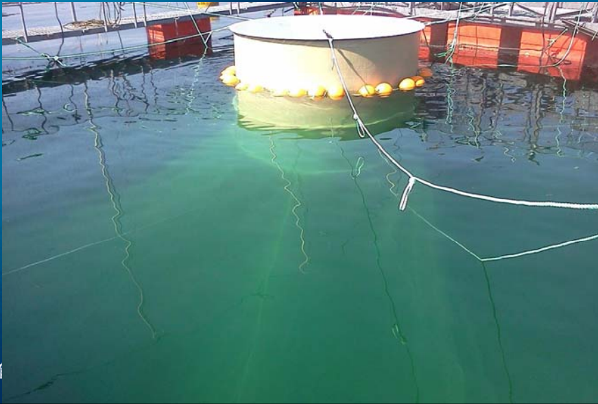
Start of trial 1 – snorkel and roof in place
