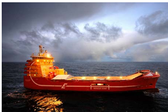
Figure 27 - M/S Viking Avant, owned by Eidesvik will be powered by a 320 kW molten-carbonate fuel cell[49]
