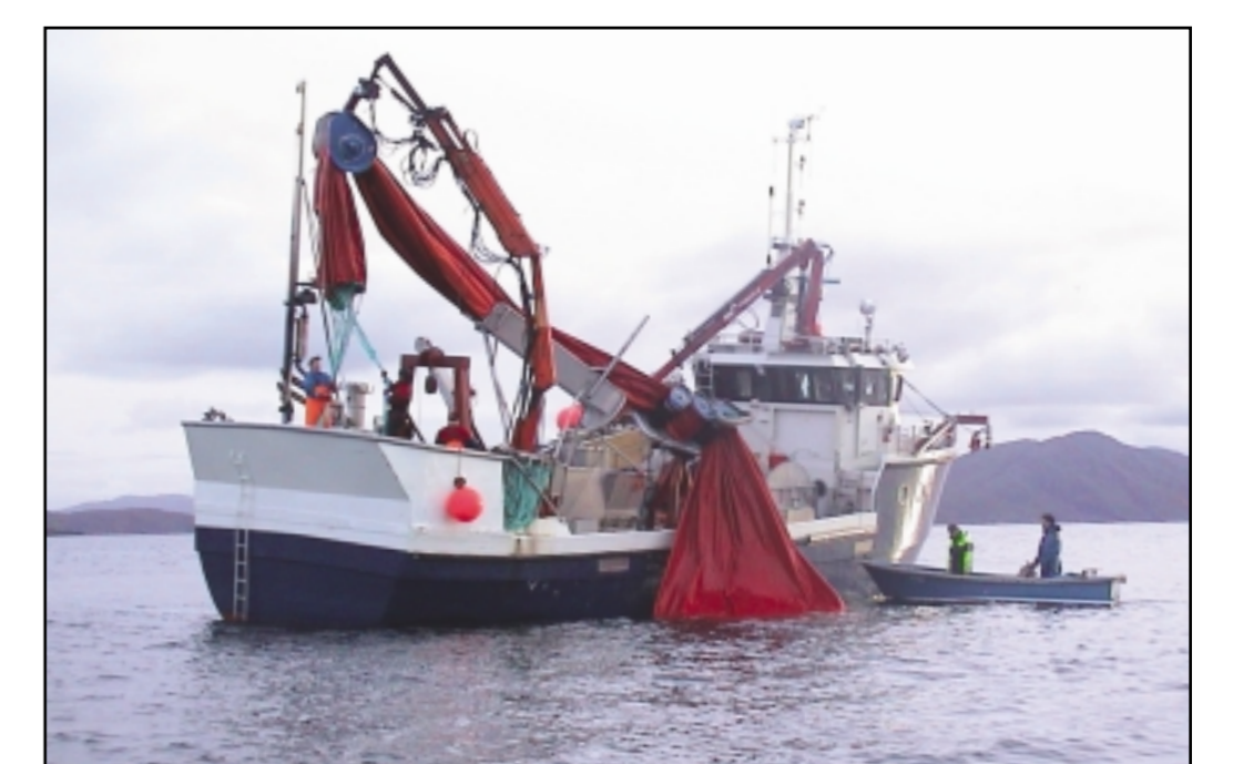
The towing cylinder is set afloat over the stern. It can be towed and kept open by the coastal seiner's life-boat, and is taken on board through the triplex.
