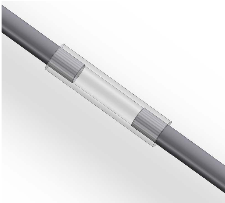
Figure 3.4: Stainless steel and acryl glass pipe combination
