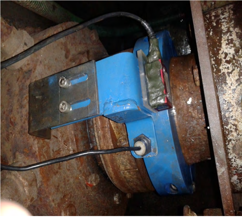
Figure 2 : Torsiometer (blue ) attached to the propeller shaft .
