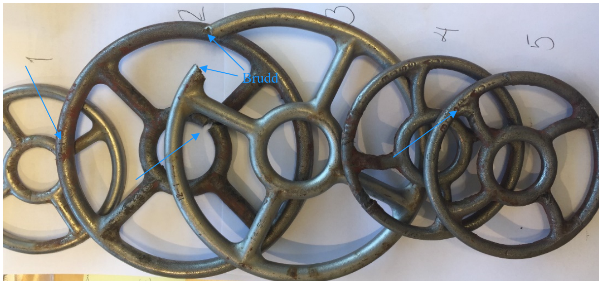
Figur 3. Korroderte stålringer mottatt for evaluering
