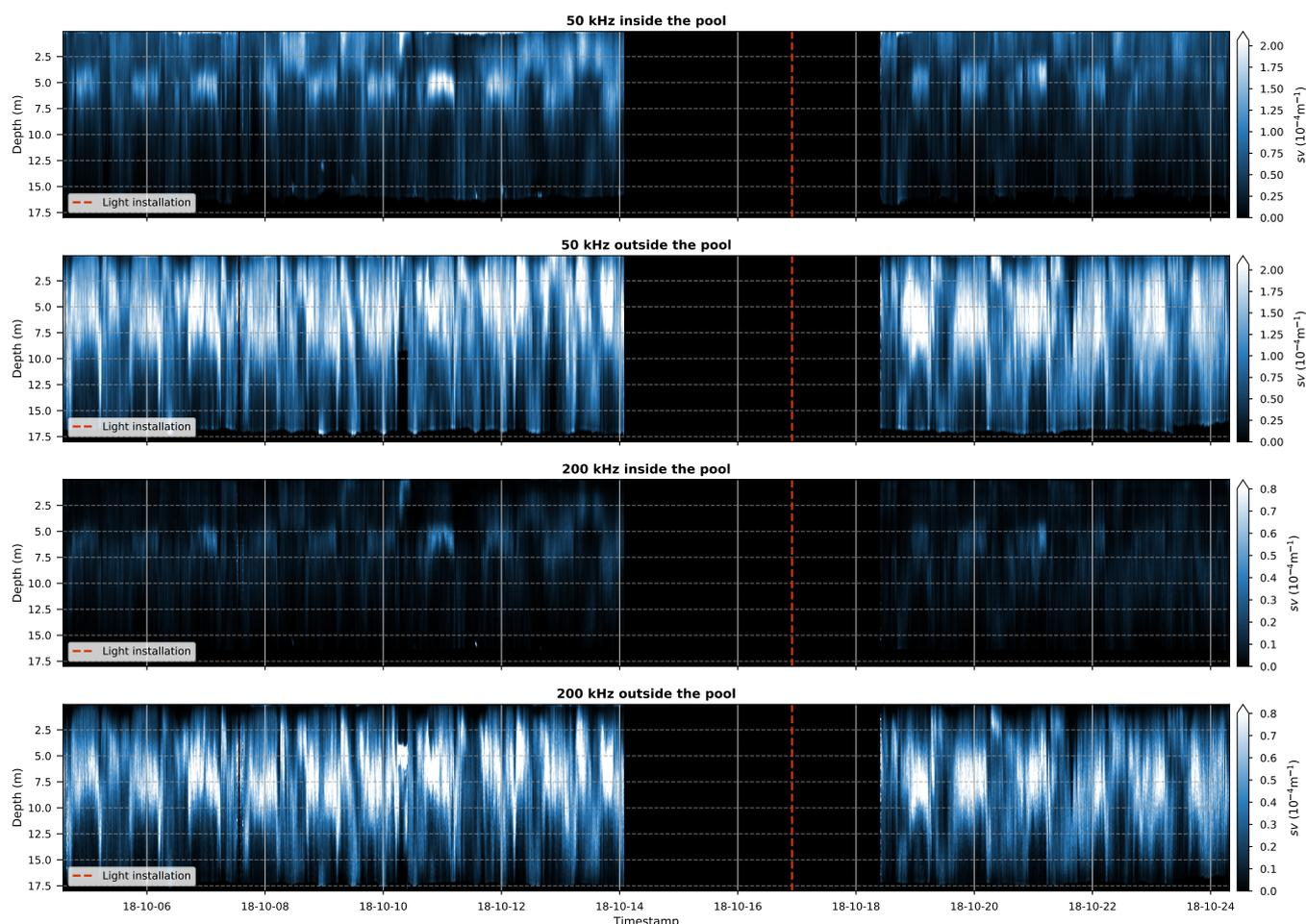
**FIG. 2: Overview echogram plot of the complete trial.** Shown are 20 minute average  $sv$  echograms for each of the involved channels. Channels with same frequency share a color scaling for easy absolute comparison. The red dashed line marks the day at which lights were installed.
